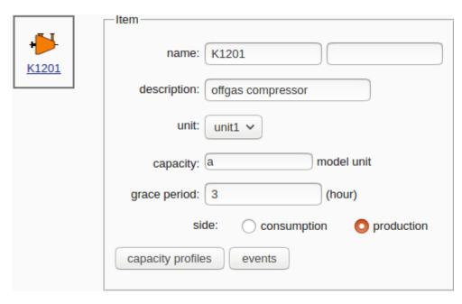
For an item with a positive grace period, its downtime does not reduce system capacity immediately, but only after the grace period has expired. For example:
